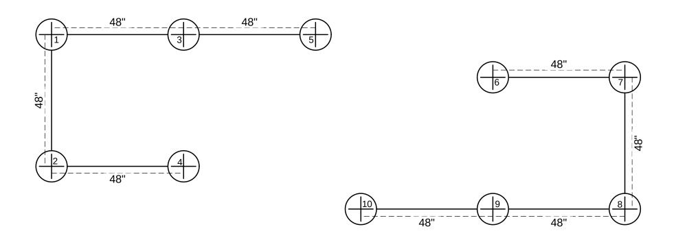
Footer Layout provided as a guide. Measurements rounded to nearest 1/2 inch. For true accuracy, please measure using equipment onsite. Equipment dimensions are subject to change without notice.
