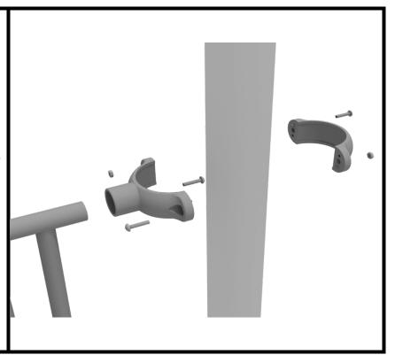
Connect the Net Climber to the designated post using four (4) 3.5-inch tube clamps.
