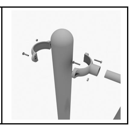
Using two (2) M10\*25 bolts, four (4) M10 washers, and two (2) M10 lock nuts, connect the guardrail to the deck. Repeat steps 2 and 3 for the other guardrail.
