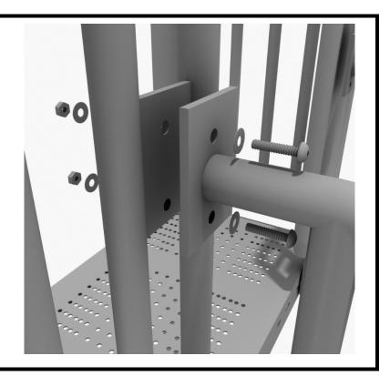
Using one (1) M10\*25 bolt, two (2) M10 washers, and one (1) M10 lock nut, attach the top of the stairway to the deck on the opposite side of the posts. Repeat this step for remaining attachment points.
