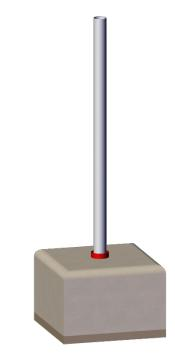
• Pour concrete into the foundation pipe, ensuring the post is straight, and allow to dry for the manufacturer's recommended amount of time.
