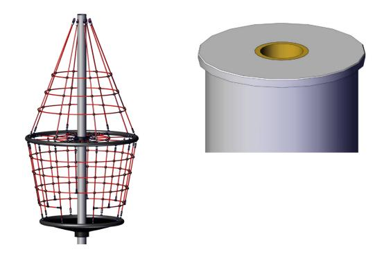
• Slide the outer post down over the inner post until the ball inside the top plate is seated into the bearing plate (you won't be able to see the bearing, but when seated properly the outer post will rotate freely). The outer post fits over the bottom friction sleeve of the inner post, and inside the collars at the middle ring and the center of the Bird's Nest.
