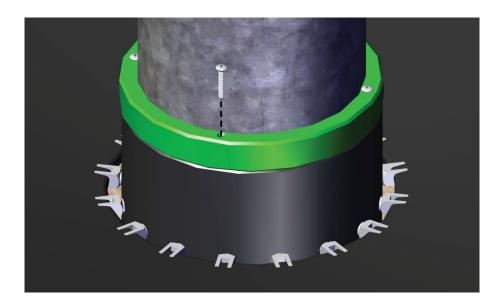
• Place the post cap over the top plate as shown, and secure with the washer and lock nut. If the threaded rod protrudes from the tightened lock nut, or if there is not enough thread, remove the post cap and adjust the height of the rod.
