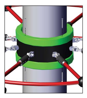
• Fit the last two gap ring sections (shown in green below) over the bottom collar at the center of the Bird's Nest. Hold the ring close against the post and top of the collar then use the remaining six Torx screws to anchor the ring to the collar.
